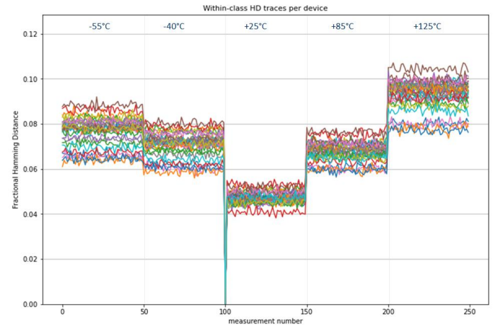
Figure 2: SRAM PUF measurements from 30 devices in UMC 65nm technology node, depicting the Within-Class Hamming Distance (WCHD) between measurements of the same device at different temperatures and a reference measurement at room temperature (first measurement at 25°C). At every temperature, 50 measurements were taken per device. WCHD levels at room temperature are between 4% and 6%. At more extreme temperatures the WCHD compared to room temperature increases up to 11%.
