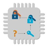
Zign 200 uses inherently random SRAM start-up values as a PUF from which the root key is generated. The root key is never stored and is only available (in volatile memory) when needed. This means the key is never present in
