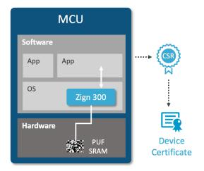
in persistent memory – not even when the chip is powered down – which raises the security significantly and eliminates the need for OTP or secure memory.
