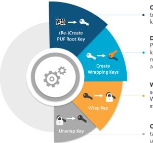
**Creates secure root key.** Uses start-up values of SRAM to create a device-unique root key. Re-creates this root key each time it is accessed – the key is never stored
